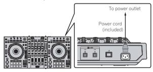
6 Press the [0] switch on this unit's rear panel to turn this unit's power on.
